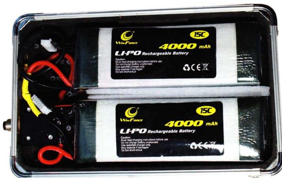
Figure 1. The power source for the author's electric bike. Two series-wired 5s LiPos from China built into a small aluminium case with a thermal fuse.
